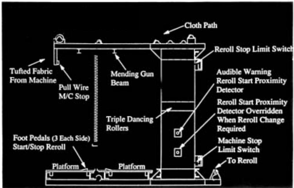
Figure 10 A modern burling frame for inspection and mending
